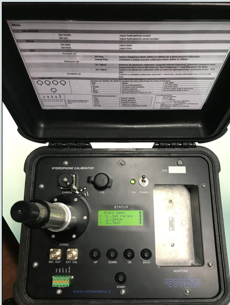
Battery operated field calibrator for Colmar GP series hydrophones. Using custom adaptors it can be used even with different types of hydrophones.
