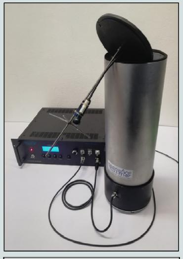
The T1 Acoustic Calibrator consists in a "standing wave tube" and provides a rapid, portable, and reliable hydrophone calibration in the low frequency range (100Hz -1.8kHz).
